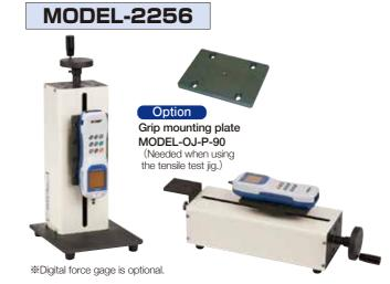
A vertical and horizontal manual handle type small stand dedicated to RZ Series and SX Series. Capable of measurement up to 500N. The gage mounting part can be moved by turning
