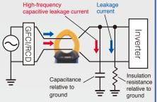
Measure leakage current at frequency characteristics that approach those of the GFCI or RCD
