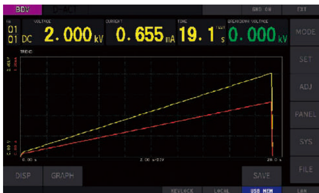
Example of continuous voltage rise test
