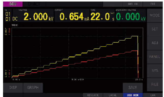
Example of stepped voltage rise testing
